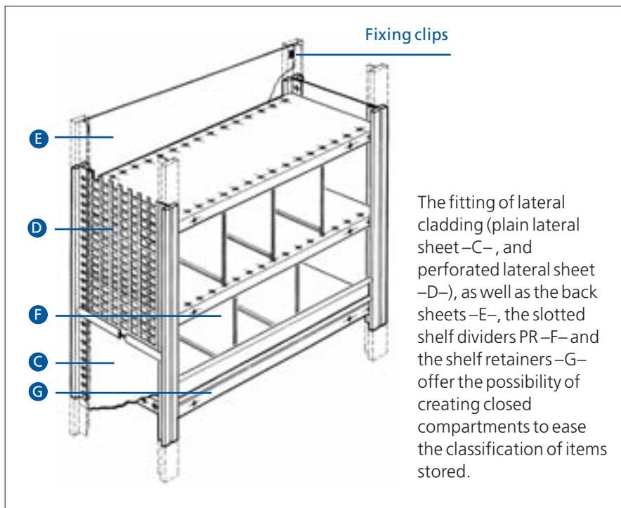
The fitting of lateral cladding (plain lateral sheet -C-, and perforated lateral sheet -D-), as well as the back sheets -E-, the slotted shelf dividers PR -F- and the shelf retainers -G- offer the possibility of creating closed compartments to ease the classification of items stored.
