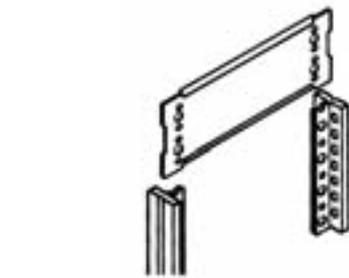
**Cross tie (2).** The cross ties are bolted to the uprights providing the shelving with transverse stability.
