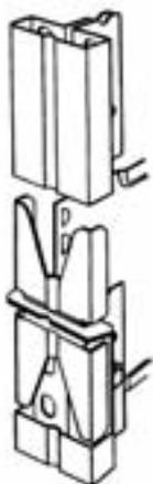
**Splice union.** The splice union PS fits into the end of the uprights permitting an extension to the height of the Shelving.
