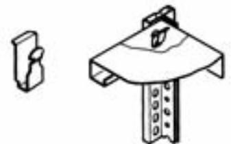
**Shelf support clip (7).** Shelves which are not supported by beams require four shelf support clips.
