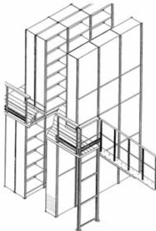
When calculating an installation with various floors in height, the number of gangways will be determined by the total height of the installation, taking into account that the recommended height between gangways ranges from 2200 to 2500 mm. The access to the different floors is by means of pre-assembled staircases. In addition, the gangways can be supplied in the form of chipboard or metallic flooring.
