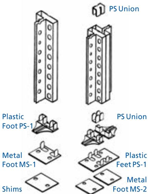
**Upright (1).** The lateral and interior sides of the uprights have slots every 25 mm in order to facilitate the insertion of various components. The PS unions are designed to join two uprights when required. The metal feet fit into the lower ends of the uprights in order to reinforce their stability on the floor.
