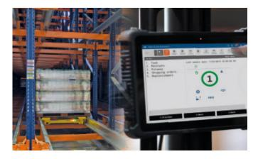
The electric shuttle is integrated with the high-density racking, which leverages warehouse space by eliminating aisles. Moreover, this solution adapts to LIFO (last in, first out) and FIFO (first in, first out) storage and extraction criteria as needed.
