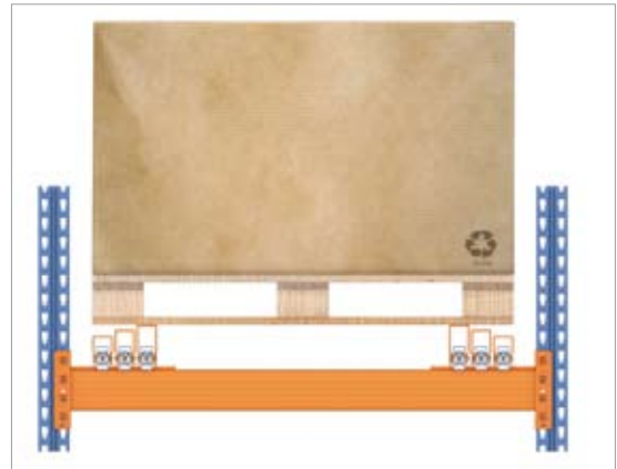
The pallet must always be properly centred.
