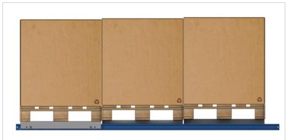
The image represents the composition of one level that is three pallets deep where we can see that there are only two sets of carriages.
