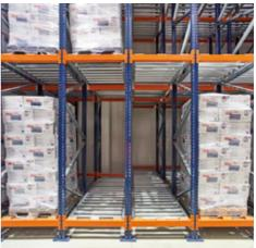
AGILITY AND SAFETY IN OPERATIONS: FORKLIFTS DO NOT HAVE TO ENTER THE RACKS AND ONLY WORK FROM ONE AISLE.
